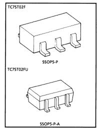
Weight SSOP5-P : 0.016g (Typ.) SSOP5-P-A : 0.006g (Typ.)
